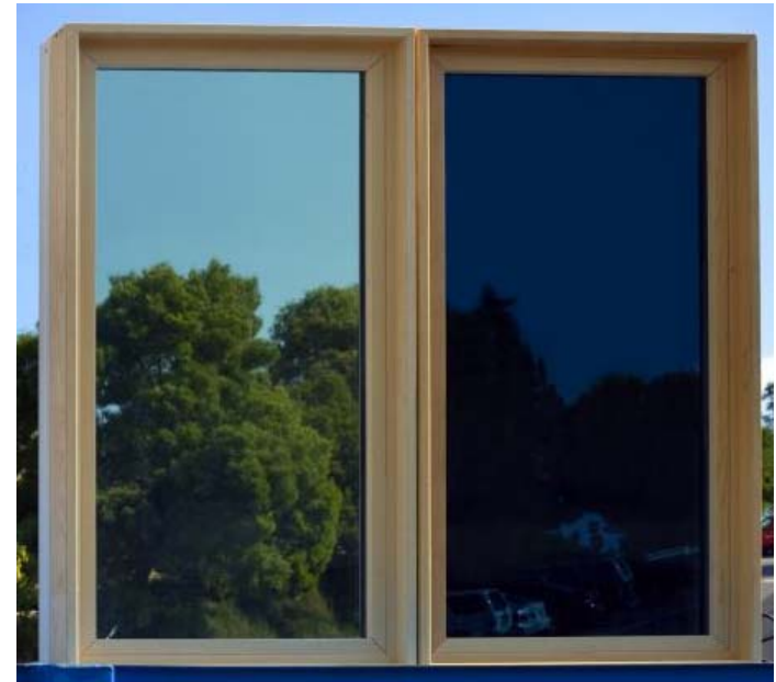
Prototype – Concept Window (Highly Insulating and Dynamic)
